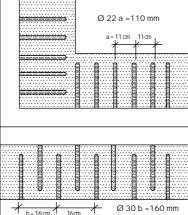
Drilling is normally done from one side only, but under certain circumstances it may be advantageous to drill from both sides - for instance in random stonework with rubble infill.
