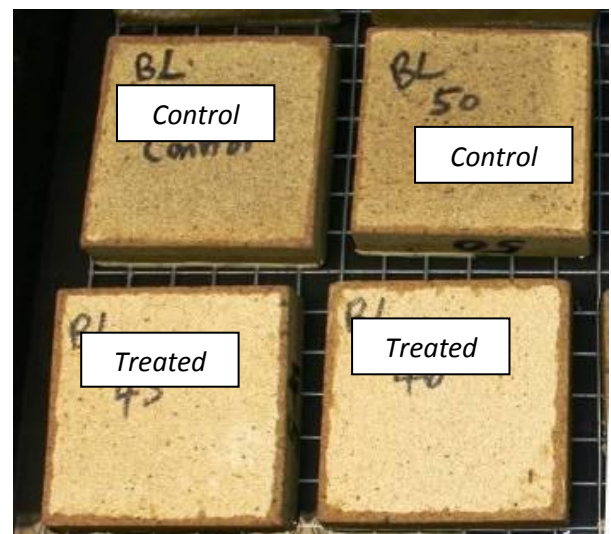
Figure 2 : Appearance of the Blaxter sandstone blocks during the water absorption test.
