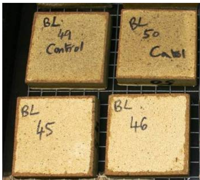
Figure 1 : Shows the appearance of the Blaxter sandstone blocks during the water absorption test.
