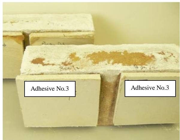
Visible salts crystallising on the brick do not transfer to the plasterboard surface
