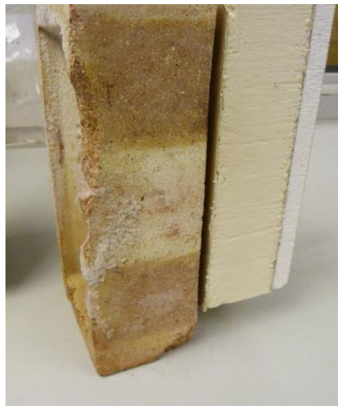
Left hand side shows the appearance during the test and the right side afterwards with crystallising salts
