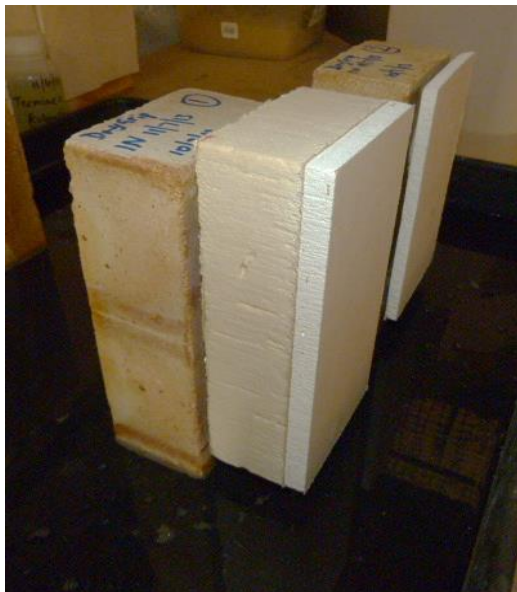
Left hand side shows the appearance during the test and the right side afterwards with crystallising salts
