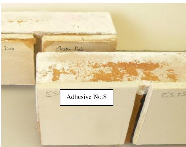
Visible salts crystallising on the brick do not transfer to the plasterboard surface
