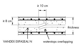
VANDEX EXPASEAL N waterstops must not be stretched during installation.
