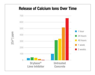
Drybase® Lime Inhibitor was shown to effectively reduce the amount of calcium released from a 3:1 sand:cement mortar block. For additional information, please refer to our research report (available on request).
