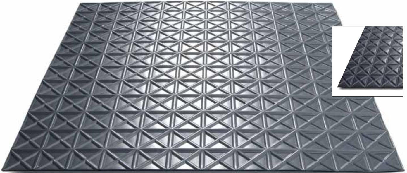
**Oldroyd Xs is a tough damp-proofing membrane that can be laid on top of damp and contaminated concrete floors, or newly laid floor slabs in above ground applications. A wide choice of flooring types can then be laid on top, for example screeds, particle board and laminated wooden flooring. Insulation can be used where required in conjunction with Oldroyd Xs, and the membrane is suitable for use with underfloor heating systems.**
