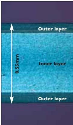
Through a microscope (above), the quality of the technology employed in the manufacturing process can be clearly seen in this cross-section.
