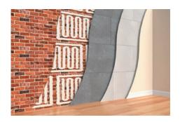
Before any works are carried out, ensure that the substrate is clean, level and suitable for application of the boards. Carry out repairs or make modifications as necessary. Remove any obstacles or fixings that might hinder application such as radiators, switches or sockets.
