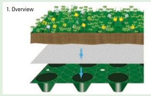
Typically the studded, perforated Oldroyd Xv20 GreenXtra membrane is laid over a suitable exterior grade flat roof waterproofing membrane, together providing roof waterproofing and drainage. Oldroyd Tp filter fleece is laid on top of the drainage layer followed by roof soil and plants.
